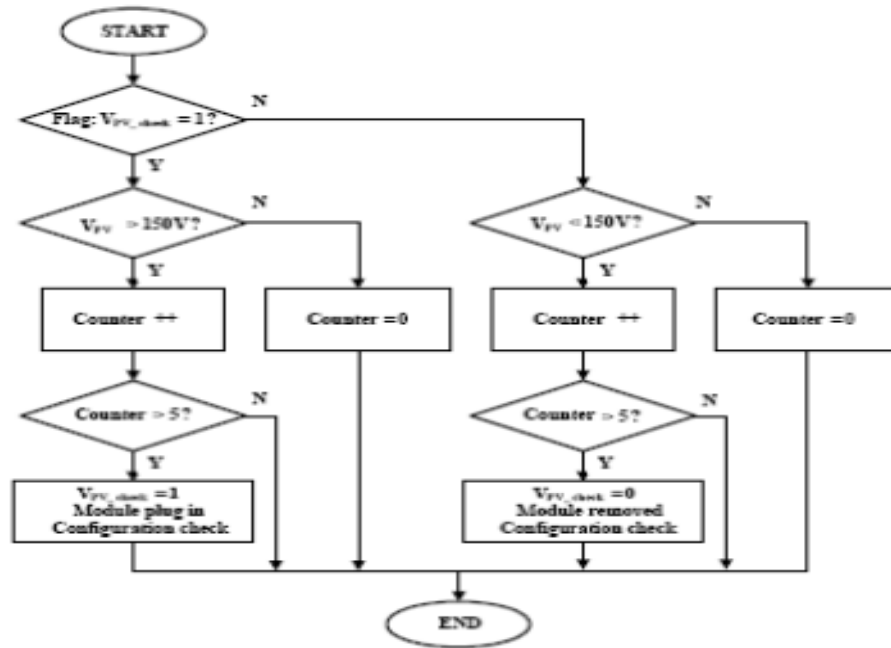
Figure 2. Online PV String Check Algorithm Flow Chart
