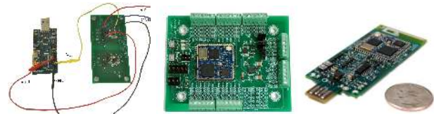
Figure 4. (a) An illustration of how simple iCount is to implement: a Maxim MAX1724 switcher is connected to a Moteiv Tmote. (b) A sensor node for environmental monitoring includes iCount support which allows expected energy usage to be compared with actual energy usage. (c) A testbed node for benchmarking applications includes iCount plus five decades of precision calibration circuitry.
