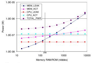
Figure 5. Logic vs. Memory Energy Trade-off. Relative contributions of energy demands due to the processor unit and the memory components, for varying memory size.
