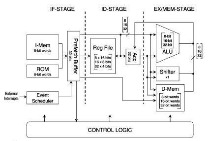
Figure 7. Sensor Network Processor Microarchitecture Overview.
