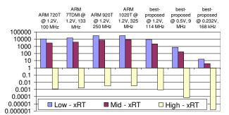
Figure 1. Performance of Sensor Network Processor Applications on Embedded Targets. xRTratings for four commercial processors and an energy-efficient design proposed in this paper at three different voltages with respect to low, mid and high-bandwidth requirements. The performance metric xRT indicates how many times faster than real time a processor performs.
