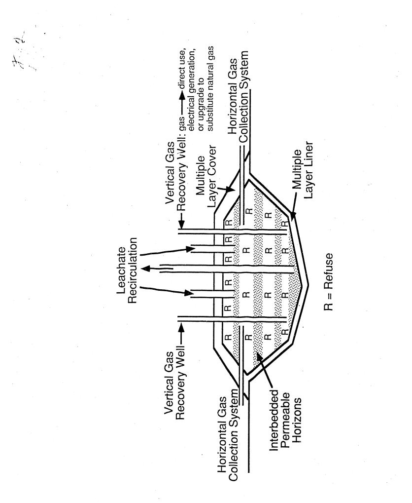
Fig. 2. Conceptual Design for a Biofill That Could Be Permitted under Subtitle D Regulations. Optimum Methane Production and Recovery with Faster Landfill Stabilization. Not Shown are Leachate and Gas Monitoring Wells/Probes.
