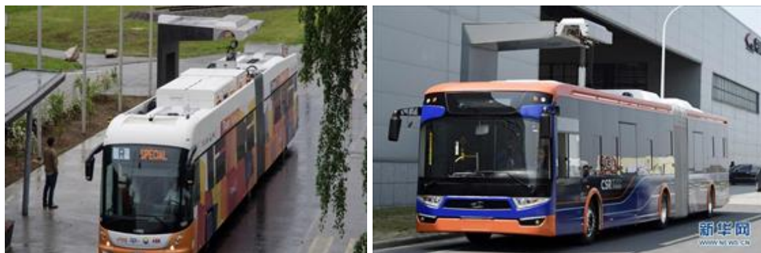
Figure 7. Ultracapacitors electrobuses of China South Locomotive & Rolling Stock Corporation.
