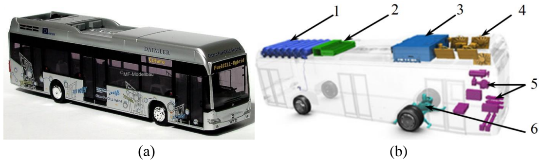
Figure 5. Electrobus Citaro FuelCell Hybrid (a) outer appearance, (b) electrobus design, (1) H 2 Tanks, (2) Battery, (3) FC System, (4) Cooling System, (5) Auxiliary components, and (6) Wheel-hub motor [39].
