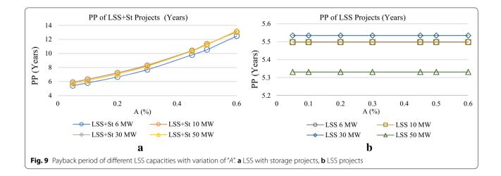
values. For A=5%, 50, 30 and 10-MW LSS projects and LSS+St projects PP have a difference of around 5 months. For 6-MW capacity, LSS and LSS+St projects PP have a
