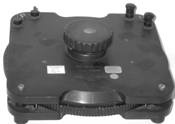
Brooks Inductometer. As late as the 1950s, students studied the theory and operation of alternating current bridges, thus becoming knowledgeable about the use of complex numbers. The Brooks Inductometer was used to produce a variable self-inductance for a single circuit or a variable mutual inductance between two circuits. Inside were four fixed coils and two coils that could be rotated with respect to them with the knob on the top. This model provided a range of 12 to 100 millihenrys. H.B. Brooks and F.C. Weaver of the Natural Bureau of Standards designed the apparatus and it cost $150 in 1920–21, when it was bought by Westminster College. (Photograph and notes by Thomas B. Greenslade, Jr., Kenyon College)
