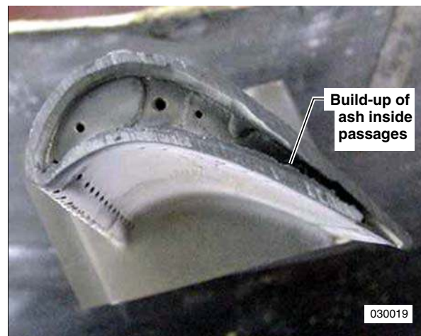
(c) Build-up of ash inside passage.
