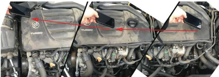
Fig. 1. The phone recorded as it was moved over the engine to provide background noise to test algorithm robustness. Engine covers were left on to minimize prep work and provide a better representative use case for in-situ monitoring.
