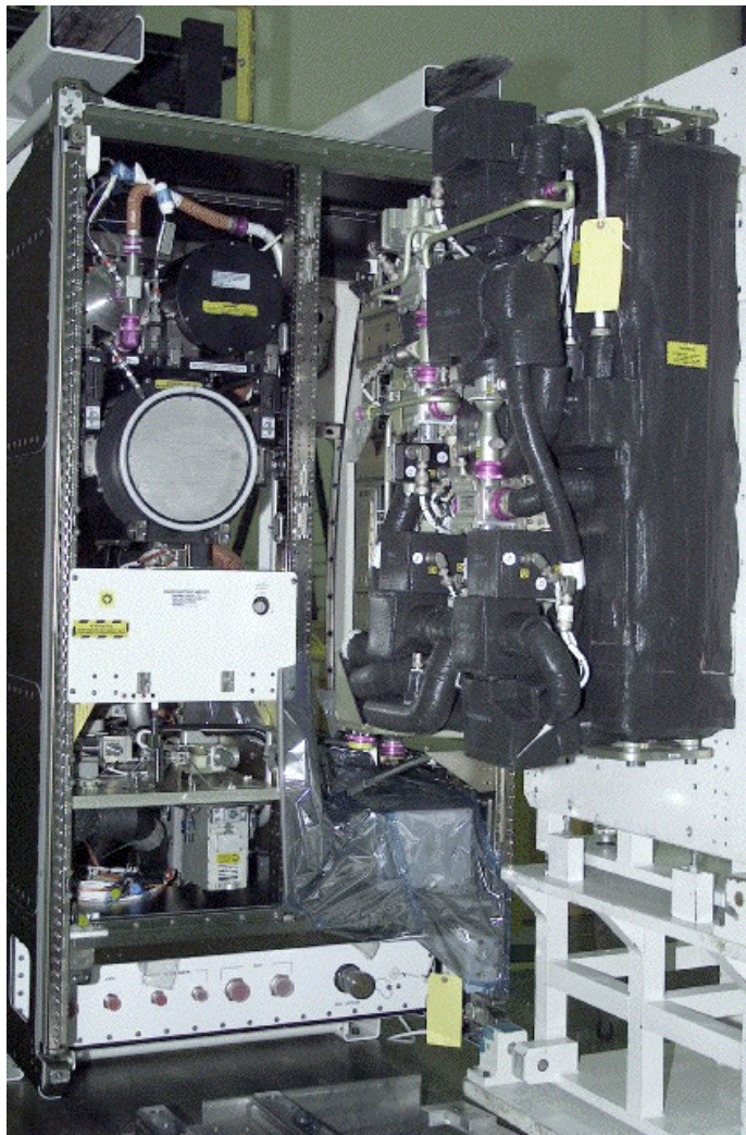
Figure 1: The four-bed molecular sieve (4BMS) carbon dioxide removal assembly used in the International Space Station
