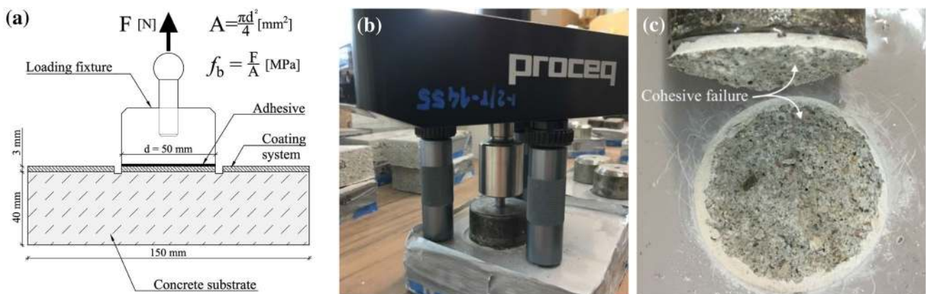
Fig. 6 The pull-off strength test (a, b) and cohesive failure (c)
