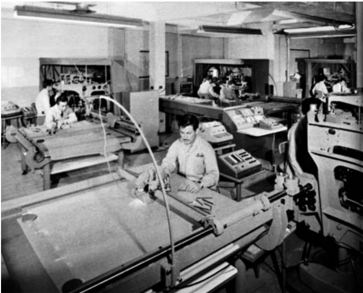
Figure 3. Mechanization of engineering projects at ICA, Aereofoto circa 1967. Photogrammetry capabilities for highway design included a punched-card machine (toward the back). (Courtesy of Fundación ICA.)
