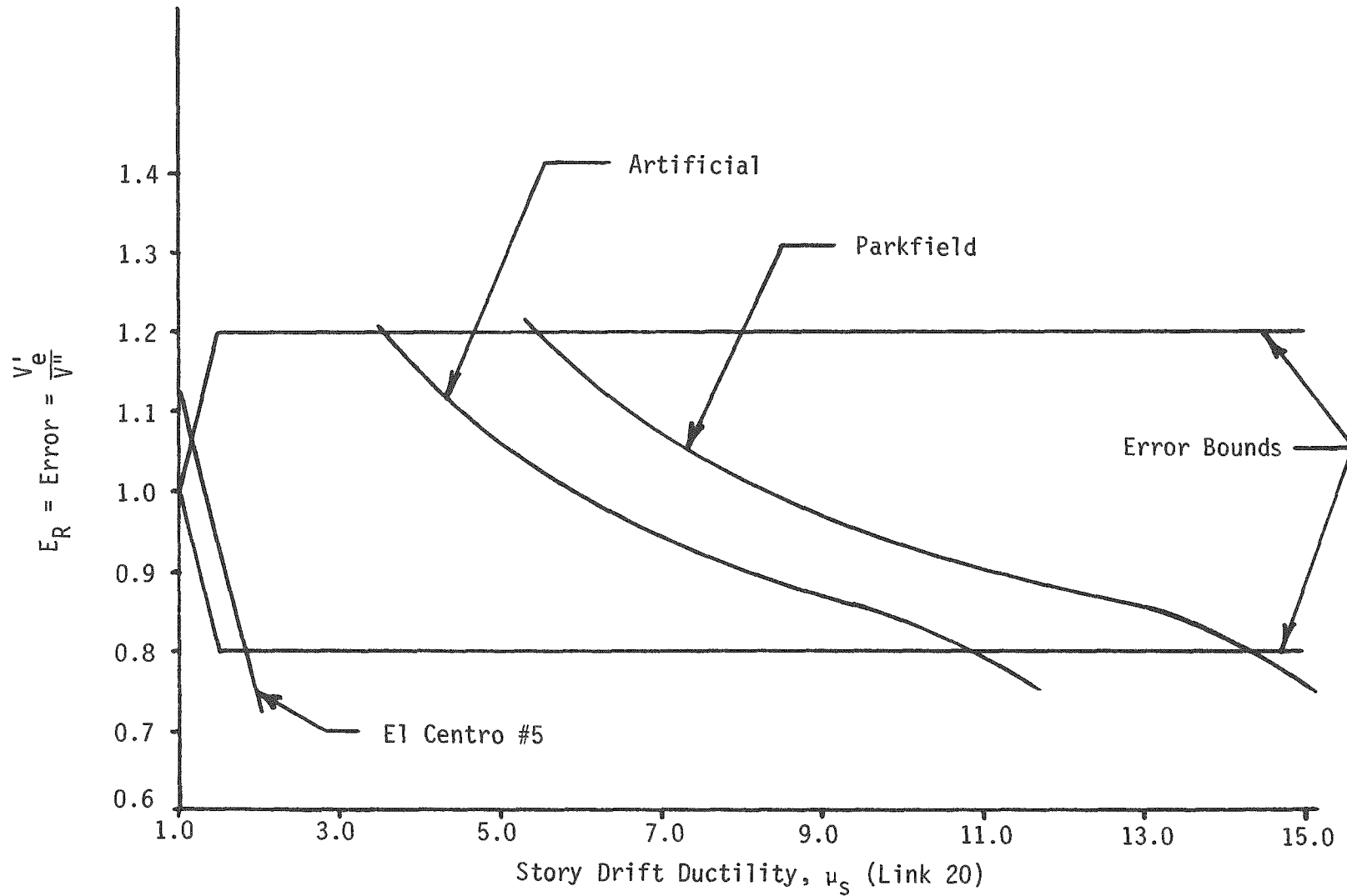
FIGURE 5-12. MODEL ERROR VERSUS STORY DRIFT DUCTILITY FOR ELEMENT 20, STIFF SOIL CASE
