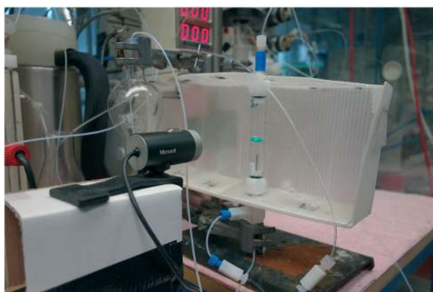
Fig. 6 An open-source machine vision system 22–25 was used to control the continuous extraction in Phase 2. The low-cost consumer web-camera detected the position of the green coloured float, sending information to a Raspberry Pi device which in turn sent commands to an Arduino board connected to a small peristaltic pump.
