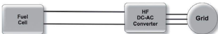
Fig. 18. A typical FC configuration with a DC-AC converter interfacing directly to the grid
