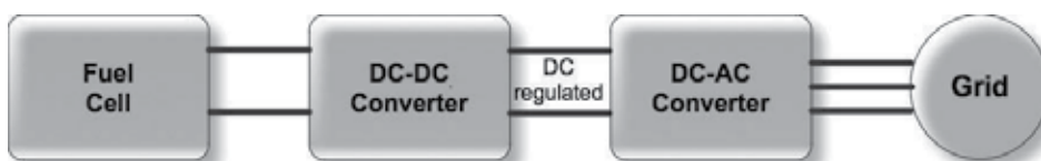
Fig. 19. A typical FC configuration with a DC-DC and a DC-AC converter
