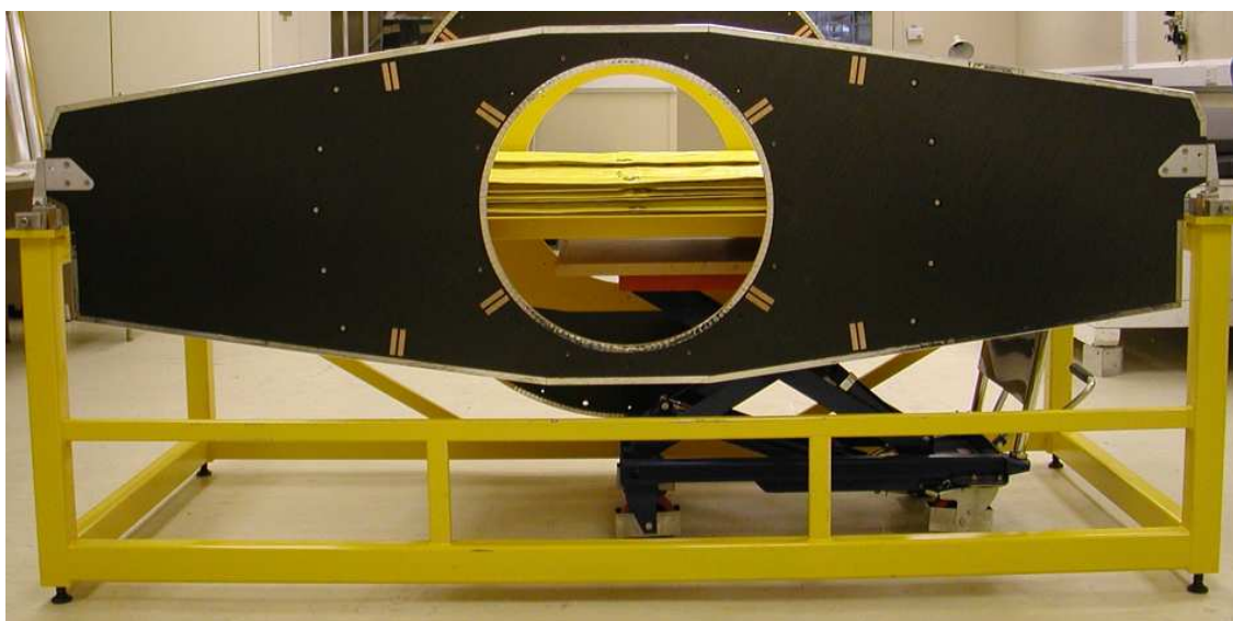
Figure 24. Front support during load testing.
