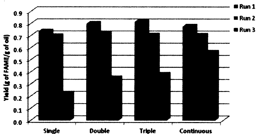
Figure 34. Effects of methanol addition on enzyme reuse from the transesterification of used vegetable oil by T. lanuginosus lipase. Reaction conditions: 1 mL used vegetable oil, 4 mL isoctane, 500 U lipase, 40 °C, stir speed 250 rpm, 3.0 mol equivalent total methanol. 130 \mu L MeOH added at t = 0 for single, 65 \mu L MeOH added at t = 0 and t = 2 h for double, 43.3 \mu L MeOH added at t = 0 , t = 1 h, and t = 3 h for triple, and 130 \mu L MeOH added over 4 h for continuous at 32.5 \mu L/h.
