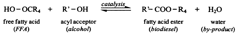
Figure 1. Production of biodiesel by (a) transesterification and (b) esterification.
