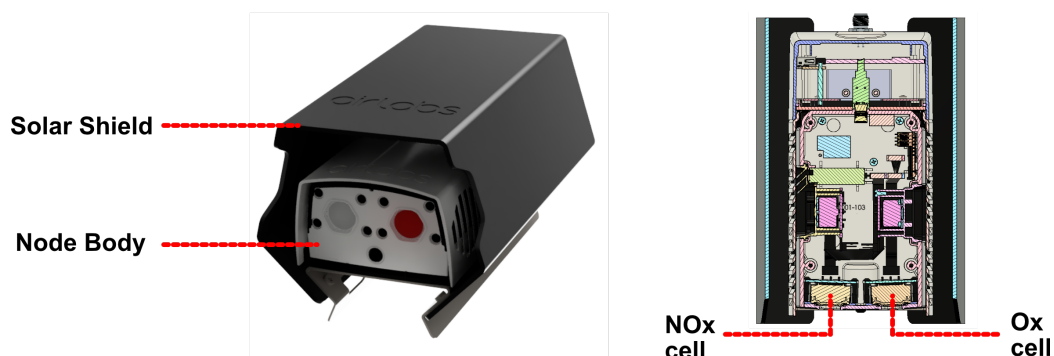
Figure 2. Gen 5 node views, node with heat-shield installed (left), and cross-section of the node with sensor locations (right).
