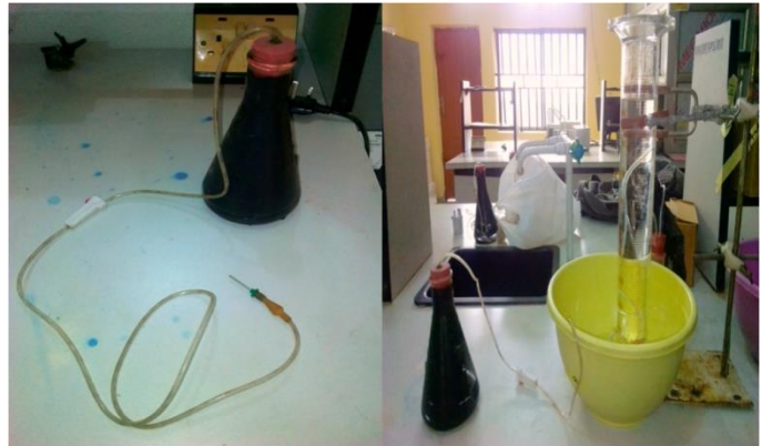
Figure 3: Biogas production and measurement set up
