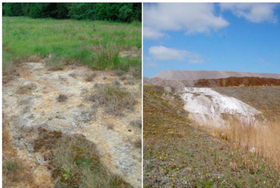
Figure 8. (left) A “hardpan” of carbonate formed on waste slag mounds at former steelworks in Consett, United Kingdom. (right) Carbonate precipitation in waters egressing from a waste landfill in Scunthorpe steelworks (photograph courtesy of Carla-Leanne Washbourne). In both cases, rainwater has percolated through the material (dissolving Ca 2+ and Mg 2+ ) and contact with DIC promotes the precipitation of carbonate.
