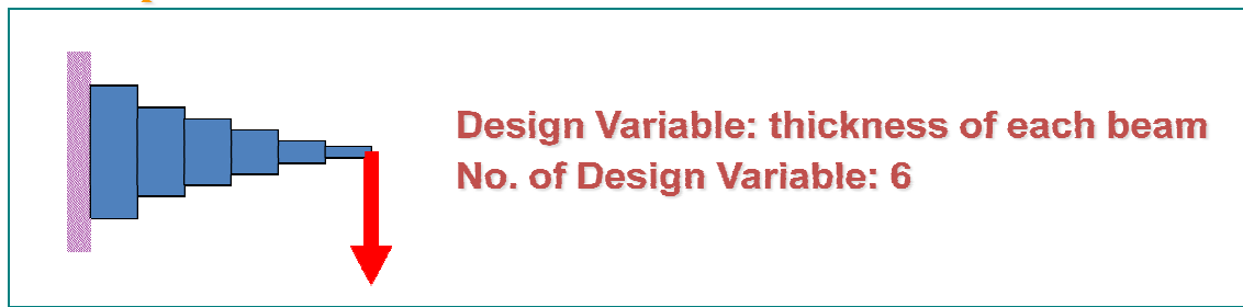
Figure 2. 4 Size optimization of beam with six elements
