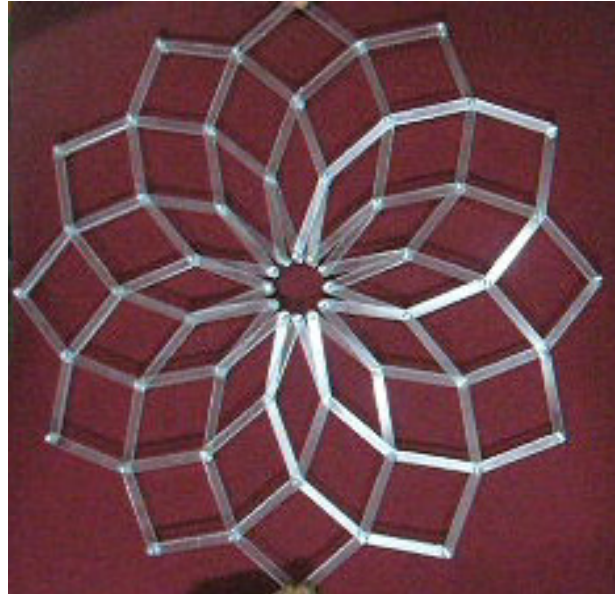
Figure 1. 4 Planer Hoberman mechanism [15]
