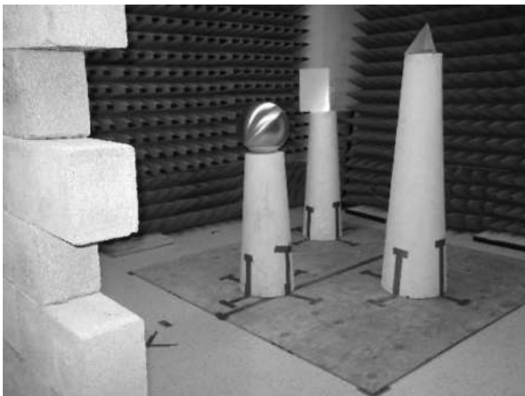
Fig. 3. Experimental setup: Calibration objects.
