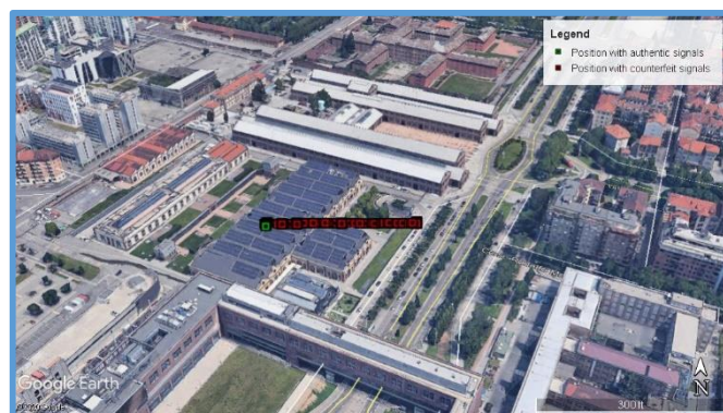
FIGURE 17°. Position obtained with authentic signals, static position at the LINKS Foundation premises roof antenna (green dots), and spoofed trajectory, moving toward East after the starting of the attack (red dots).
