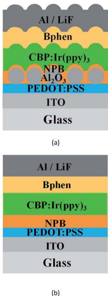
Fig. 1 The schematic diagrams of (a) the embossed PHOLED and (b) the planar PHOLED.
