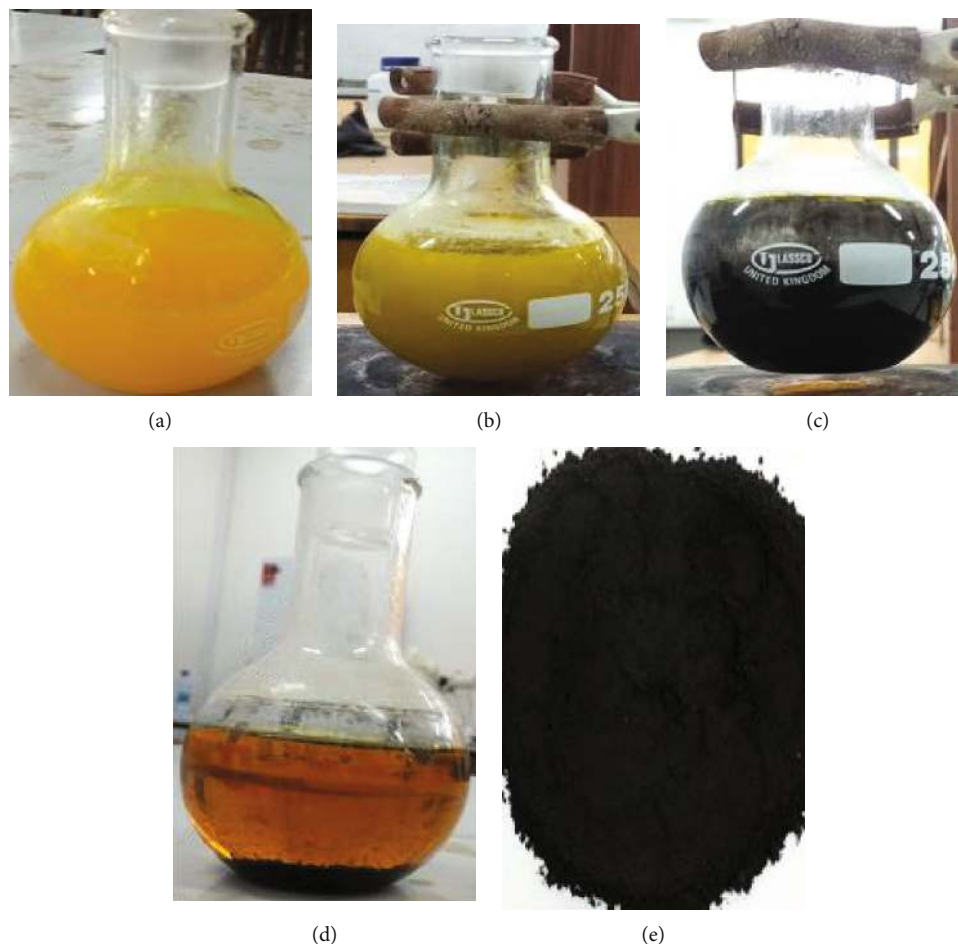
FIGURE 1: The color change observed during the stepwise synthesis of bismuth sulfide.
