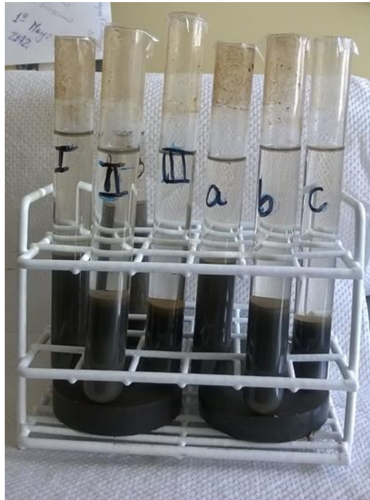
Figure 4: Demulsification after six months (magnetically assisted).
