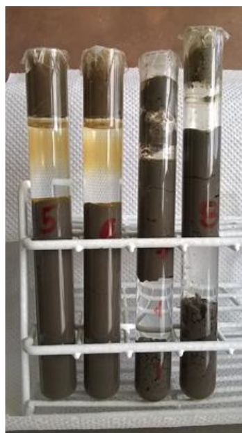
Figure 6: Behavior of selected MNPs (left) versus conventional flocculant (right)
