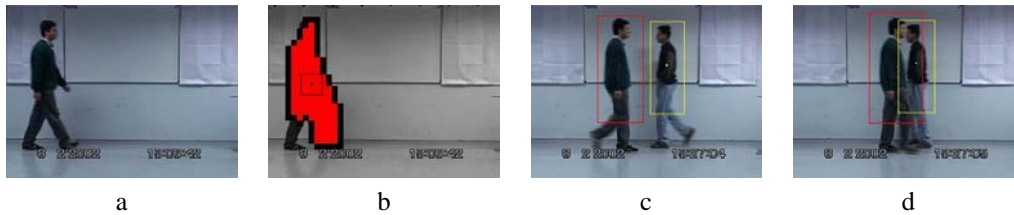
Figure 2: Motion- and proximity-boxes. Frame (b) shows CoM and motion-box marked against the segmentation result for the single object present in frame (a). Frames (c) and (d) of the persons sequence containing two objects (about to merge) show the respective CoMs and proximity-boxes
