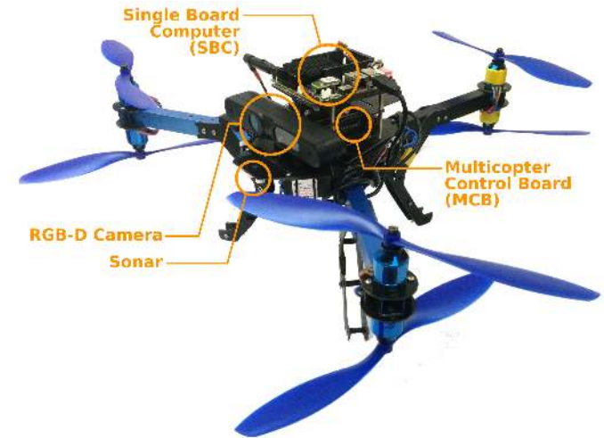
Fig. 1. Hexacopter enhanced with an on-board computer and extrospective sensors: an RGDB-D camera for visual navigation and a sonar for altitude control.
