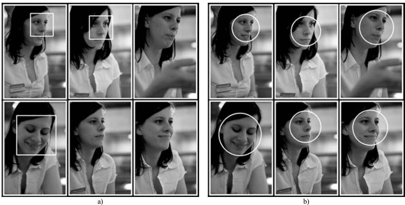
Figure 3. Visual examples of face detection algorithm quality: a) Viola-Jones algorithm; b) CEDT approach
