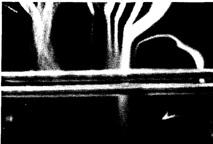
Fig. 32: 0.83 s After switching on -20 kV .
