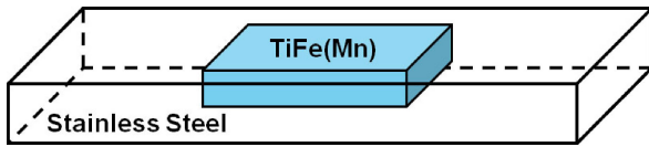
Fig. 2 TiFe(Mn) sample embedded in stainless steel sheet.
