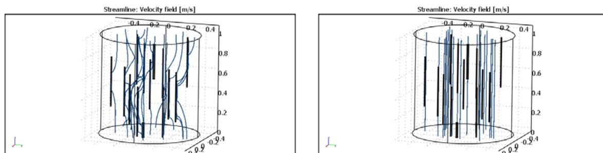
Fig. 3. Illustration of the flow pattern in the soil column for two applied boundary pressures. (a). 0.30 m, (b).  $-0.20$  m.
