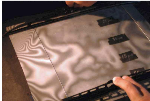
Fig. 4: First prototype in use over a curved panel. In this case the adaptation needs a right alignment and the tensile stress on the foil is somewhat inhomogeneous. It gives poorer results than the tripod approach. We may appreciate moiré fringes in the central area due to a non-perfect adaptation disturbing a reliable detection of surface deviations.
