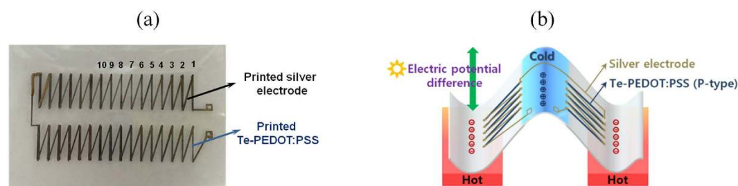
Figure 5. (a) Image of the planar thermoelectric generator consisting of 32 legs arranged in two rows and (b) schematic diagram of geometry of the invented thermoelectric generator and the generation of electricity.
