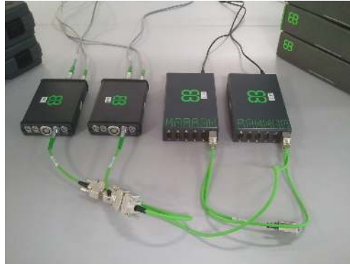
Figure 6.1: Replicated test bed comprising 4 ECUs.
