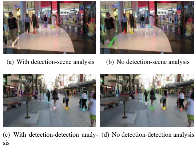
Figure 1. Results of multiple hypothesis tracking with/without enhancing detection model. (a)(b):detection-scene analysis, which penalizes detections or tracks which do not fits the scene model, helps to solve false tracks with high confidential false positives. (c)(d):detection-detection analysis, which models the correlation between close targets, helps to increase the recall, especially when detections are overlapped.
