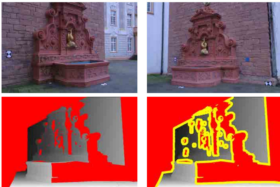
Figure 1.4: Matching with occlusions. Top row: Two images from wide-baseline stereo, with large occluded areas. Bottom row: On the left, we show the ground truth depth map, from the viewpoint of the rightmost camera. Occlusions, determined from ground truth visibility maps, are shown in red. On the right, we dilate the occlusion map by 25 pixels, and plot the result in yellow. We can think of these as the coordinates of the pixels that will be affected if we compute descriptors over a circular area of radius 25 pixels, as occluded areas creep into their domain—pixels closer to occlusion boundaries will suffer more. As the baseline increases, more and more pixels suffer from this problem: over 30% visible pixels in this case.
