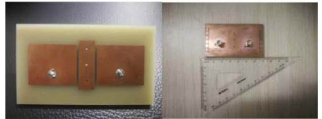
FIGURE 19. The prototype of proposed antenna: top view (left) and bottom view (right).
