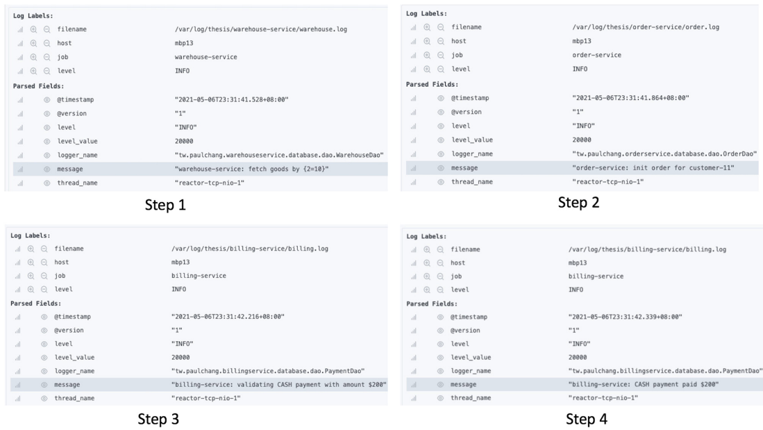
Figure 7. Steps 1–4 in version 1 (deploying standard saga pattern).
