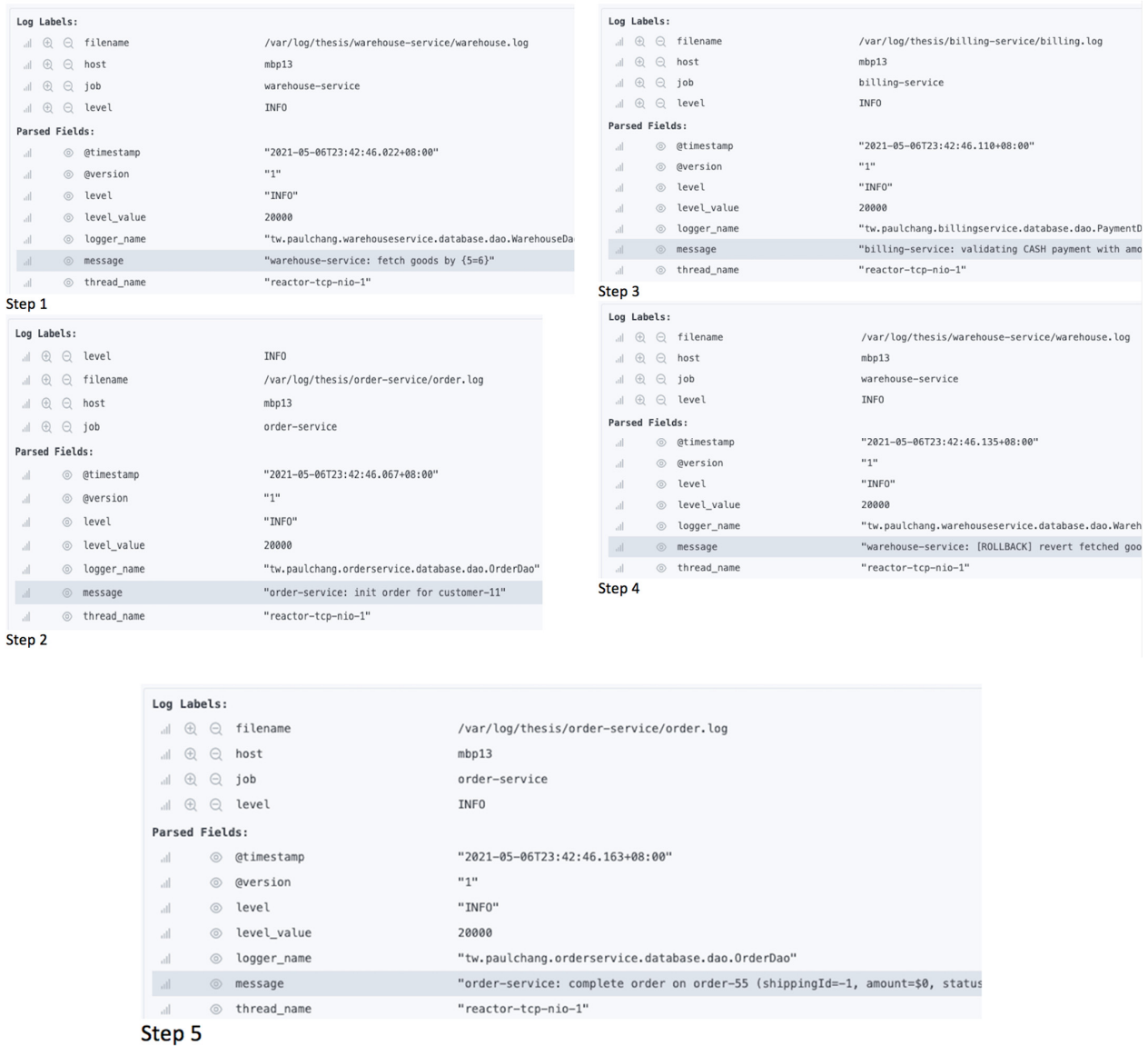
Figure 11. The Steps performed by version 1 (deploying standard saga pattern) when an exception has occurred.
