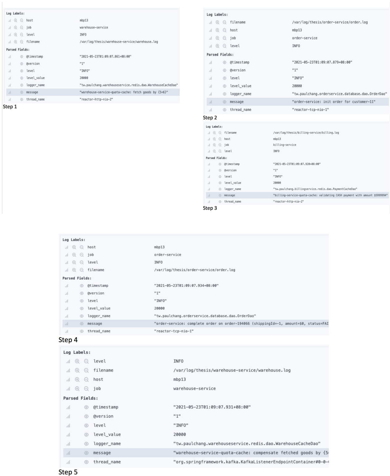
Figure 12. The Steps performed by version 2 (deploying enhanced saga pattern) when an exception has occurred.
