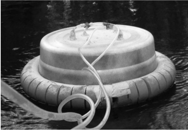
Figure S2. Picture of floating chamber, tubing, and listed dimensions.
