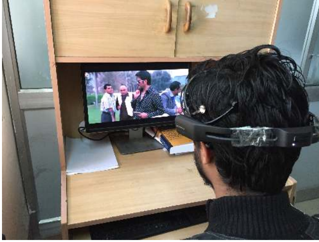
Fig. 5 A subject watching a video while wearing EPOC Emotive Device (EEG Device setup).
