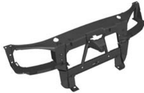
Figure 4-1: Front subframe system of Ford Mondeo
