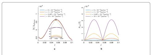
**Fig. 7** The effect of the coupling term  $\gamma$  on **a** the macroscopic rate term  $\dot{c}$  and **b** the macroscopic equivalent stress  $\bar{\sigma}_{eq}$ . The equivalent stress is calculated as  $\bar{\sigma}_{eq} = \sqrt{\bar{\sigma}_{11}^2 + \bar{\sigma}_{22}^2 + 2\bar{\sigma}_{12}^2}$
