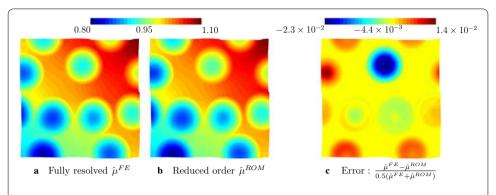
**Fig. 4** Chemical potential field  $\hat{\mu} = \mu/\mu_{\text{max}}$  in the microscopic domain at time step  $\hat{t} = 250\Delta\hat{t}$ . **a** Fully resolved finite element solution  $\hat{\mu}^{FE}$  **b** reduced order solution  $\hat{\mu}^{ROM}$  and **c** the relative error with respect to their average  $\frac{\hat{\mu}^{FE} - \hat{\mu}^{ROM}}{0.5(\hat{\mu}^{FE} + \hat{\mu}^{ROM})}$
