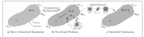
**Fig. 1** Steps involved in the development of the enriched continuum formulation: first, performing computational homogenization, the solution of a highly heterogeneous problem also known as the direct numerical simulation (**a**) is replaced by a two-scale macro and microscale coupled problem (**b**), next model reduction is performed at the microscale yielding an enriched continuum formulation (**c**)
