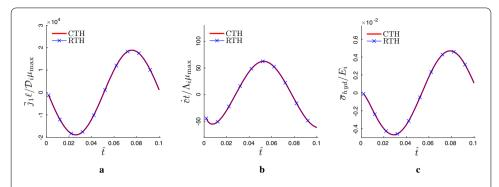
**Fig. 6** Comparison between the macroscopic quantities computed with the conventional computational homogenization (based on the fully resolved microscale RVE analysis), shown in red, and the reduced order homogenization, shown in blue. **a** Macroscopic mass flux  $j_1$  in  $\boldsymbol{x}_1$  direction, **b** macroscopic concentration rate  $\dot{\bar{c}}$  and **c** macroscopic hydrostatic stress  $\bar{\sigma}_{hyd} = \frac{\bar{\sigma}_{11} + \bar{\sigma}_{22}}{3}$
