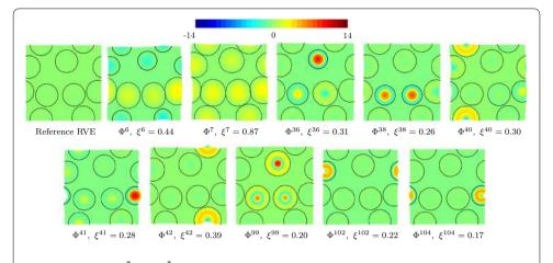
**Fig. 3** Eigenvectors  $\stackrel{*}{\Phi}_{\mu}$  and  $\stackrel{*}{\Phi}_{\mu}$  are shown in a coupled manner: the color map indicates the chemical potential value and the corresponding mechanical modes are indicated by the geometry change (swelling or shrinkage) of the inclusions. The displacement field is scaled 5 times relative to the reference configuration. The quantitative contribution  $\xi^k$  of the mode is defined in Eq. (116)
