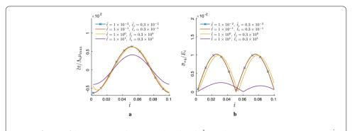
**Fig. 8** Influence of the microscopic characteristic length scale  $\hat{\ell}$  on **a** the macroscopic concentration rate  $\dot{\bar{c}}$  and **b** the equivalent macroscopic stress  $\bar{\sigma}_{eq}$
