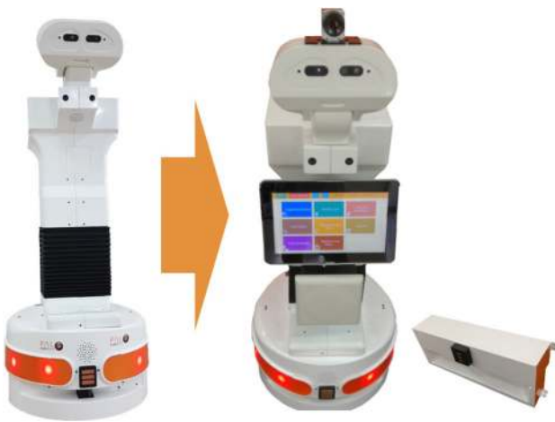
Fig. 3 Evolution of TIAGo Iron to the ENRICHME version
