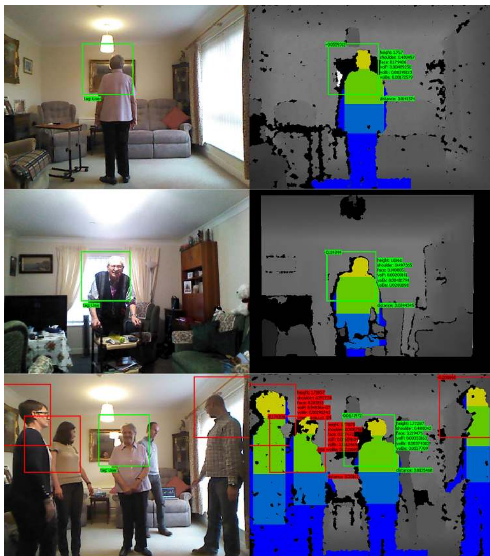
Fig. 24 The ENRICHME robot can successfully recognize the correct user in challenging situations such as non-frontal views (top row), occlusions (middle row) and multiple people presence (bottom row)
