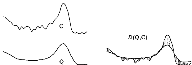
Figure 3. The intuition behind the Euclidean distance. The Euclidean distance can be visualized as the square root of the sum of the squared lengths of the gray lines.
