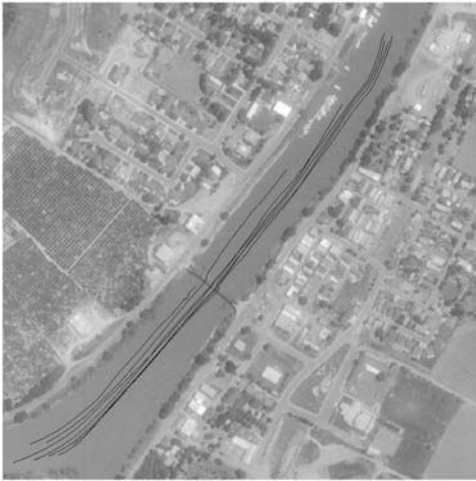
Fig. 7. An example of drifter trajectories extracted from GPS measurements in the Sacramento River on November 16th 2007.
