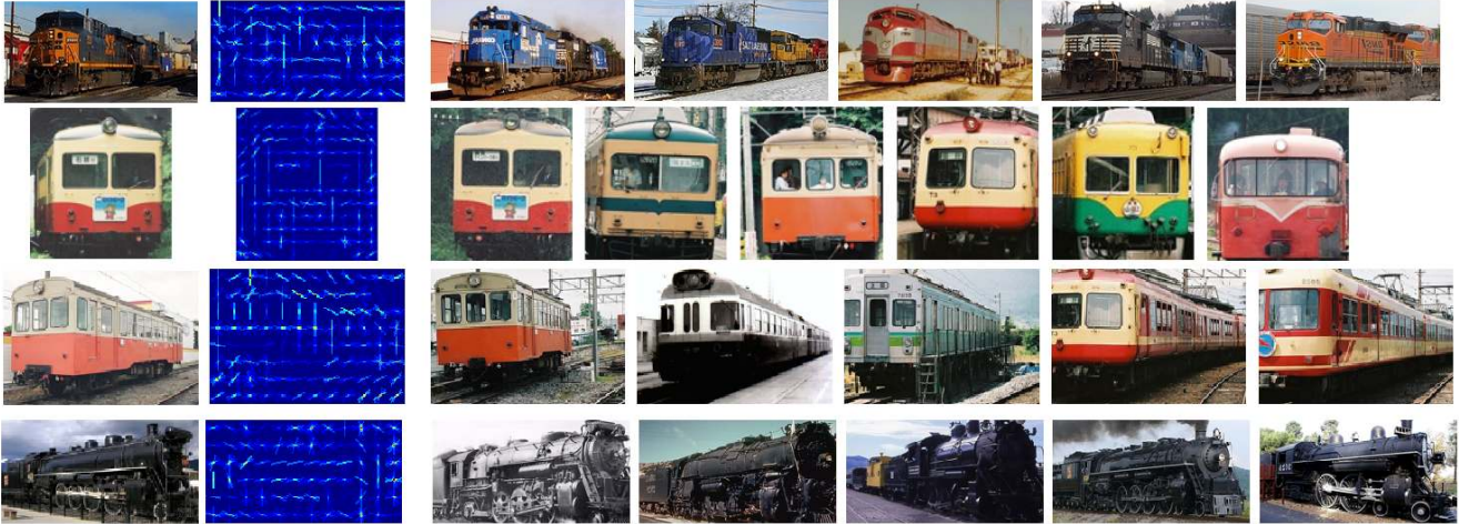
Figure 4. Exemplar-SVMs. A few “train” exemplars with their top detections on the PASCAL VOC test-set. Note that each exemplar’s HOG has its own dimensions. Note also how each detector is specific not just to the train’s orientation, but even to the type of train.
