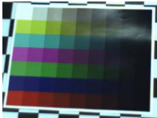
Figure 2: A sample camera image of the color calibration pattern in Figure 1 (left).
