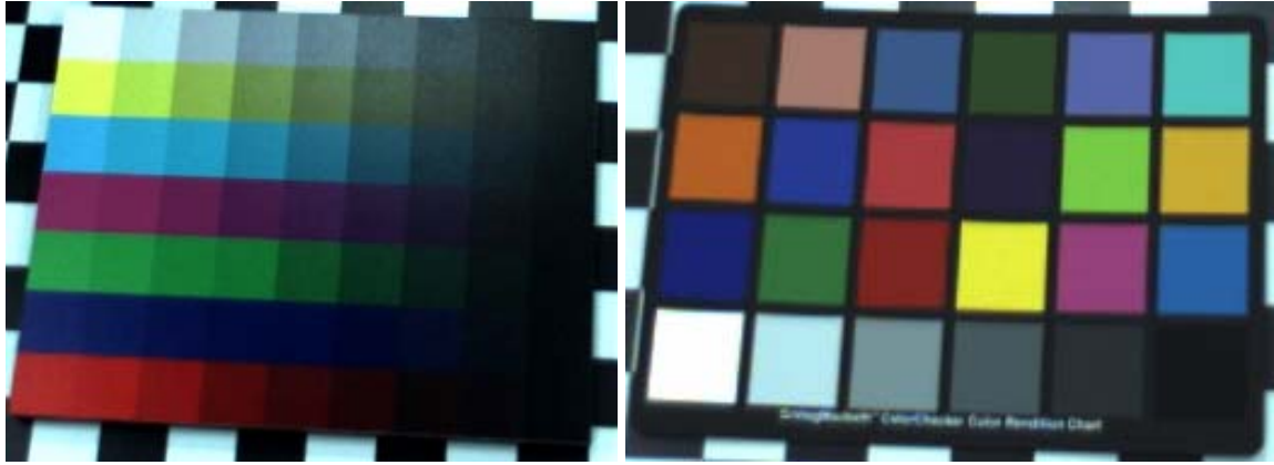
Figure 3: A sample camera image of the mounted color calibration pattern, and an image of the GretagMacbeth™ color target.
