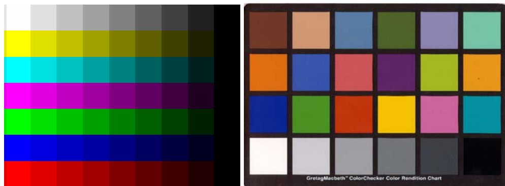
Figure 1: A color calibration pattern, and a professional color target from Gretag Macbeth™.
