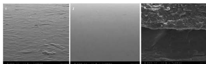
FIGURE 9 - SEM of a cross section of HPMC capsule surface (I), Gelatine capsule surface (J), and HPMC capsule surface coated with Eudragit S 100 (K).
