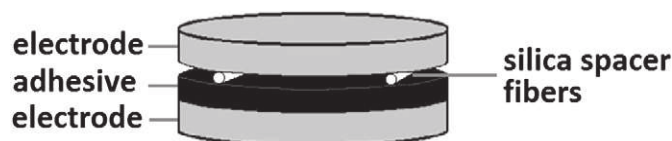
Fig. 1. Sample configuration including “air gap” for TSC experiments.
